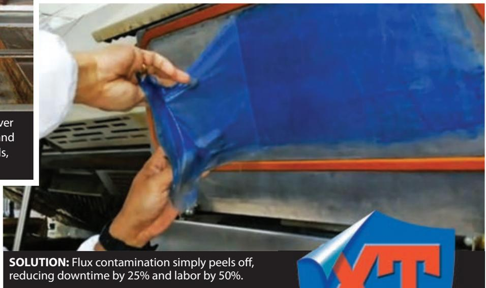
**SOLUTION:** Flux contamination simply peels off, reducing downtime by 25% and labor by 50%.
